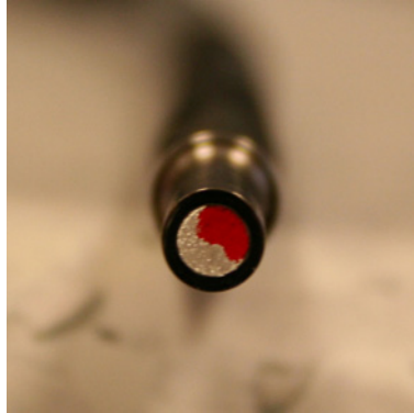
Figure 4.14: Illustration of how the fiberoptical cable splits the light into the two ends. In order to see the split, one end was pointed at a red object, while the other end was pointed towards a bright white surface. The cable can either be used with one input and two outputs, or alternatively with two inputs and one output, e.g. if two pulsers were to be connected to one MAPD in order to test the recovery time of the detector.
