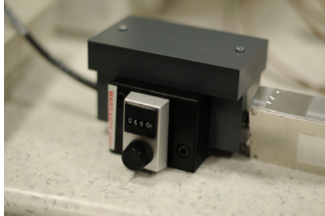
Figure 4.7: The monochromator with a plastic adapter attached. The box connected on the right is the LED pulser, the black wire to the left is the fiberoptic cable.
