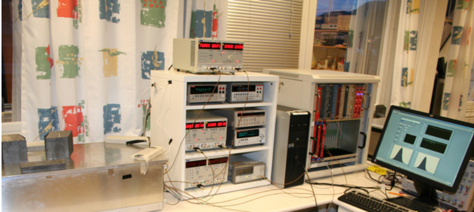
Figure 4.1: Image of the entire lab setup. The large aluminium box to the left is the black box, upon which a few lead weights are placed.
