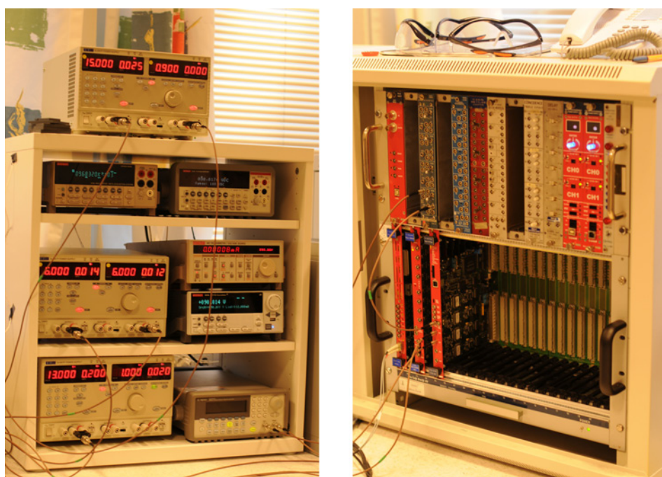
Figure 4.5: The image to the left shows the device rack, while the image to the right shows the NIM rack (top) and the VME rack (bottom).
