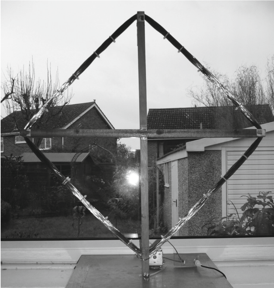
Fig. 9.1. The VLF loop antenna. It is a square with 400-mm-long sides and made up from 125 turns of enameled copper wire. There is a tuning capacitor on this one, which is not needed for this project.
