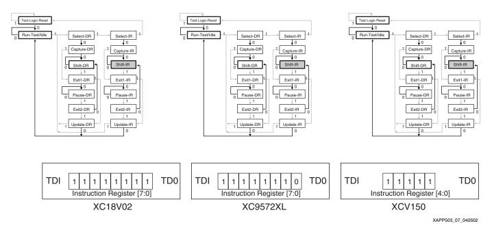
Figure 4: TAP Controller State Diagrams and IR Contents After Shifting the IDCODE Instruction
