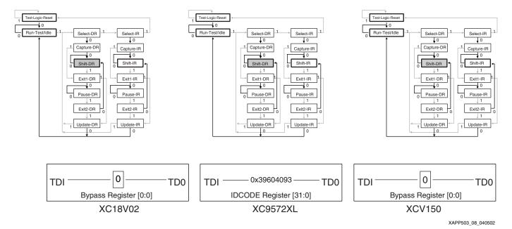
Figure 5: TAP Controller State Diagrams and DR Contents after Shifting the IDCODE and BYPASS Instructions
