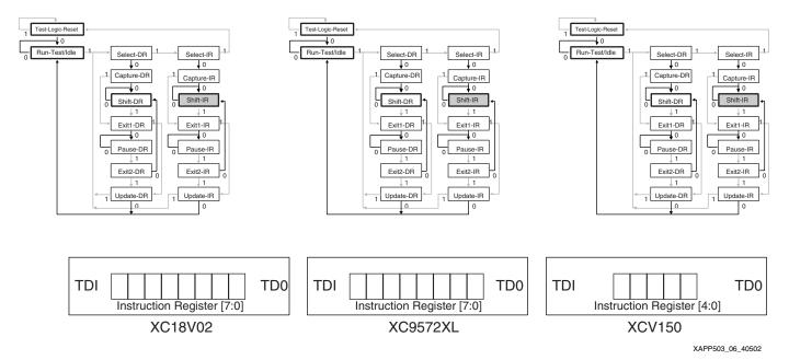
Figure 3: TAP Controller State Diagrams and IR Contents Prior to IR Shift
