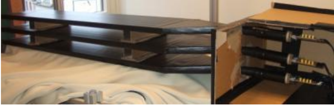
Figure 4.4: Efficiency test set-up: Three scintillators on top of each other with PMTs inside a light-proof box.
