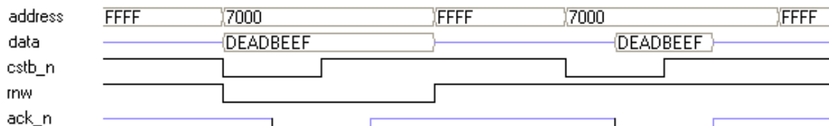
Figure 3-5: DCS bus protocol. First 0xDEADBEEF is written to register 0x7000, and then it is read back afterward (From simulation).
