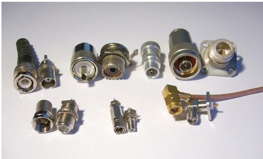
Fig. 5.12. Common RF connectors. From top left : BNC plug, BNC socket, PL259 plug and matching SO239 socket, UHF "TV" plug, N plug, N socket. From bottom left : F plug, F socket, SMB plug, SMB socket, SMA plug and SMA socket. Note that most types come in variations such as straight or angled and are available for different sizes of cable. There are also 50 and 75 \Omega impedances in some types. SMA plugs come in normal and inverted pin types.
