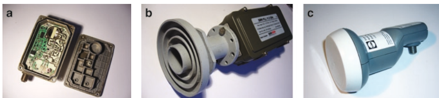
Fig. 10.2. (a) The LNB circuit. This kind of circuit is difficult to make at home. Note that the cover has built-in shielding walls to isolate various parts of the circuit. (b) LNB with a \text{c120} feed horn used on concentric dishes. (c) A European Universal LNB used on offset dishes.
