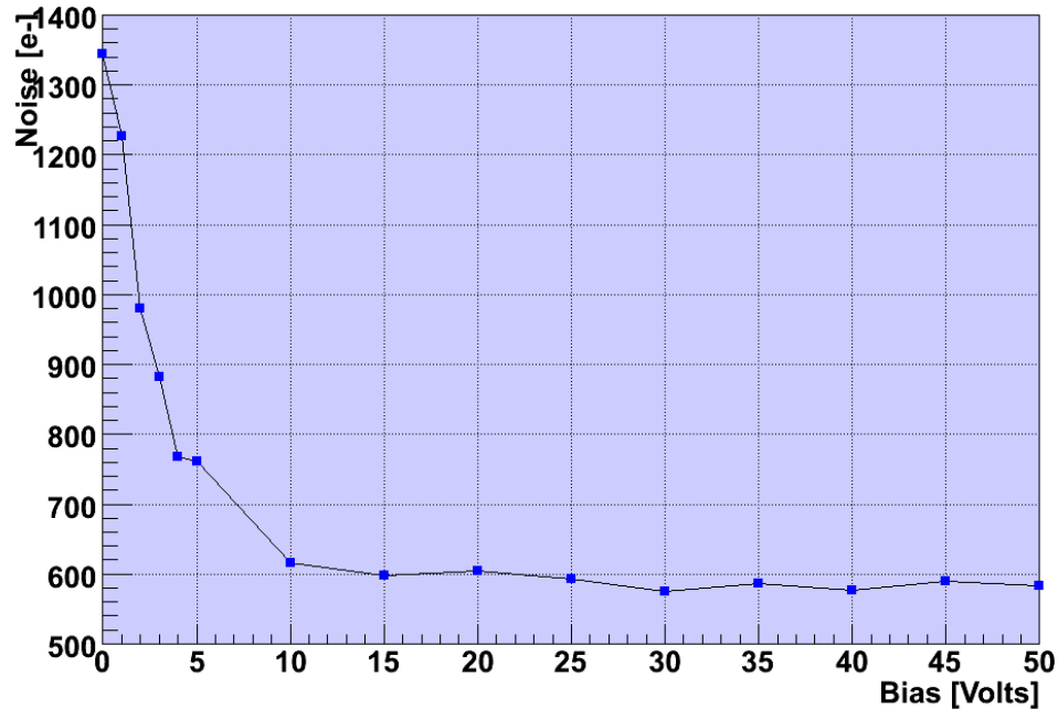
Figure 6.14: The mean noise as a function of reverse bias voltage.
