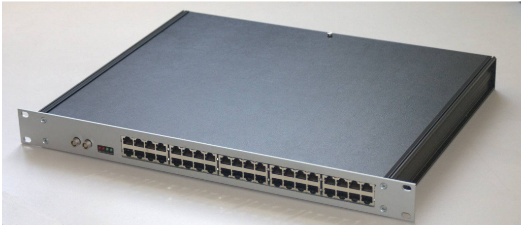
Figure 3.2: Picture of the Busy Box in a one unit 19" rack case. (Photo: C. Soos)
