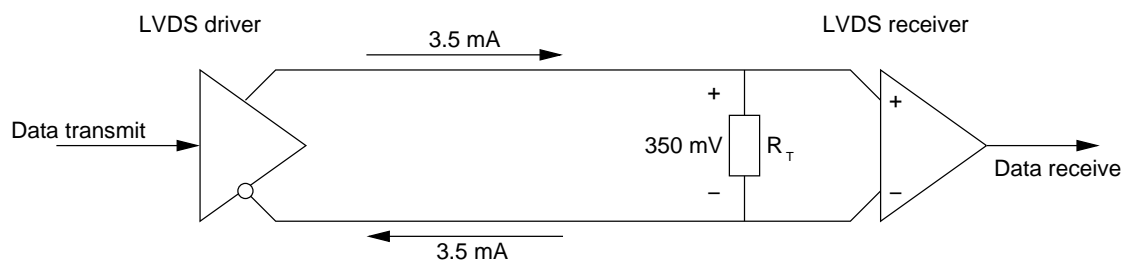
Figure 4.1: Standard point to point LVDS Application.
