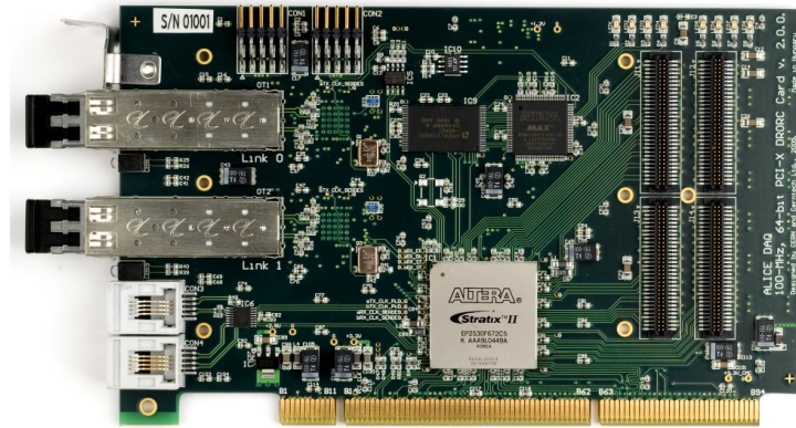
Figure 2.4: Picture of the D-RORC with two optical transceivers (SIU/DIU) and two LVDS ports.
