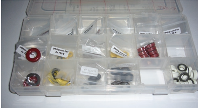
Fig. 8.8. Toroidal inductor cores. Powdered iron types are usually color coded. Ferrites are normally black .
